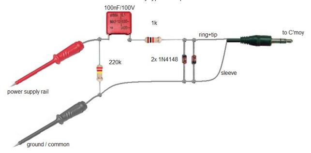
This circuit has a much higher impedance and goes lower in frequency range as well.
