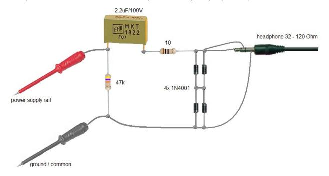
The headphone is connected in parallel to 4 diodes of which 2 of those are in anti parallel.
